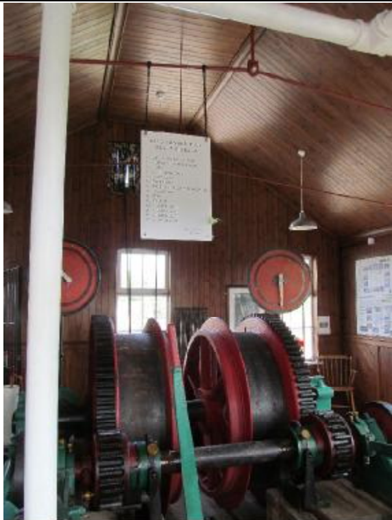
Winding gear in King Edward Mine
