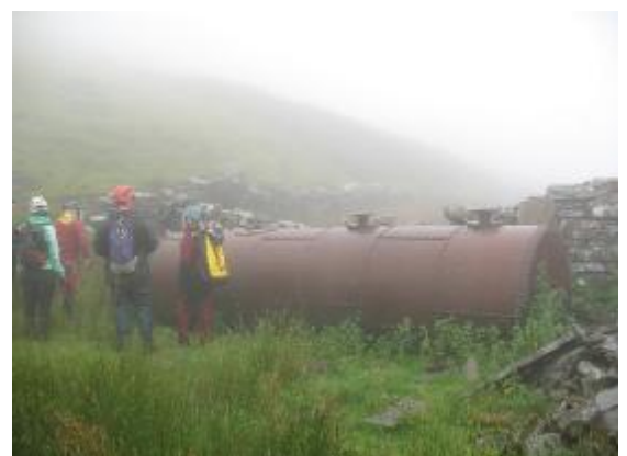
Above: Lancashire boiler at Pant Mawr mine (note Welsh weather!).
